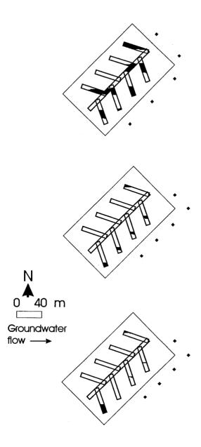
Figure 2. Releases (shaded) from which contaminant plumes were not detected in Networks 1 (top), 2 (middle), and 3 (bottom); diamonds depict monitoring wells.
